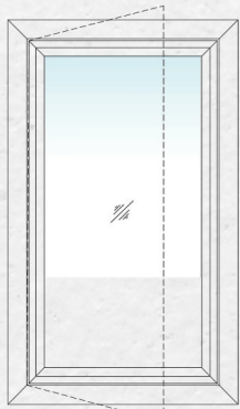
SINGLE SHUTTER OUTSIDE OPENING SIDE HUNG WINDOW
